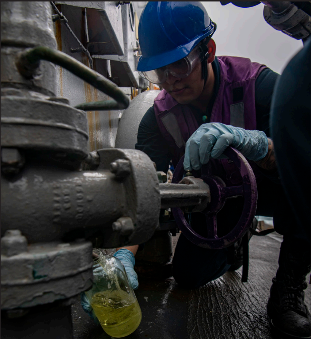
U.S. Navy photo by Mass Communication Specialist 3rd Class Brianna Walker SOUTH CHINA SEA— Gas Turbine Systems Technician (Mechanical) 3rd Class Gabriel Silva, of Hesperia, Calif., takes the midpoint sample of JP-5 fuel aboard the Arleigh Burke-class guided-missile destroyer USS Sterett (DDG 104) during a replenishment-at-sea with the Lewis and Clark-class dry cargo and ammunition ship USNS Richard E. Byrd (T-AKE 4), Jan. 4, 2025. The Carl Vinson Carrier Strike Group is underway conducting routine operations in the U.S. 7th Fleet area of operations.
